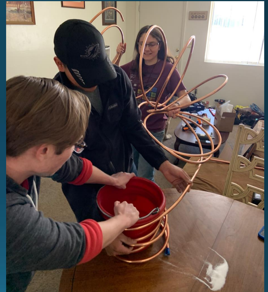
Figure 7: Coiling the Heat Exchangers
